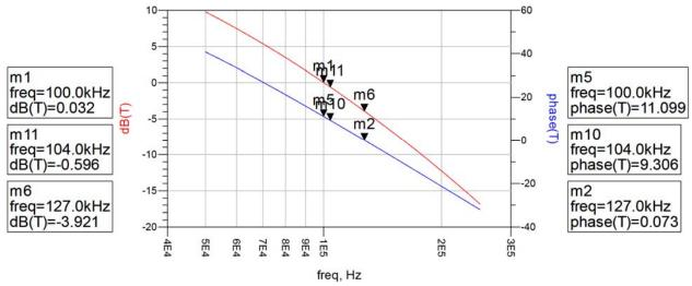
The bandwidth and phase margin are seen as 100kHz and 11.1 Deg while the gain margin is seen at 127kHz and -3.9dB. A selected point between the two indicates -0.6dB and 9.3 Deg at 104kHz.
