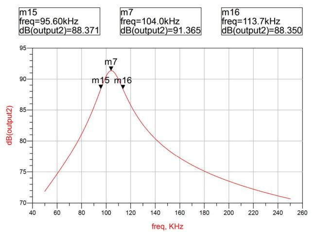
The Q of the output impedance is 104kHz/(113.7kHz-95.6kHz) or 5.76, almost identical to that determined from the length vector. Again this does not reflect the bandwidth, gain margin or phase margin, but the least stable point, as represented by the point closest to the singular unstable point, 1,0.
