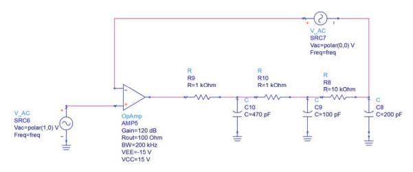
Three copies of a simple opamp circuit are used to allow simultaneous simulation and display of Bode plot forward gain and output impedance. The Bode plot is the traditional assessment, while the forward transfer and output impedance are both non-invasive measurements.
