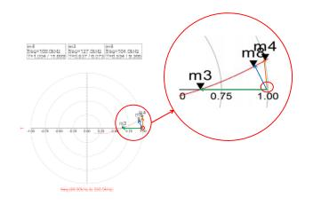
From the polar plot we can evaluate the distance from the singular unstable point 1,0 to each of the three selected data points. We can also evaluate the length of the distance as
