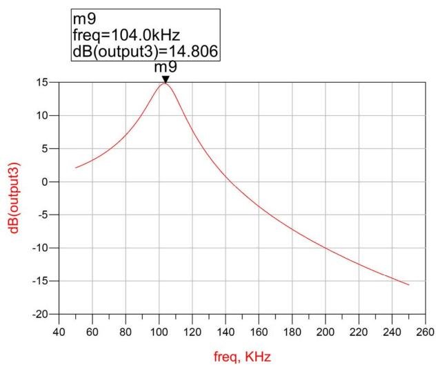
The forward gain reflects a peak with a magnitude of 14.8dB (magnitude of 5.5) at 104kHz, which is the point closest to 1,0 and is not representative of either the phase margin or the gain margin, nor does it coincide with the bandwidth of 100kHz.
