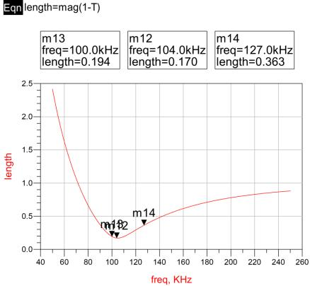
This plot shows the distance from the singular unstable point, 1,0, to the gain curve. The three selected frequencies are identified showing that the point at 104kHz is the closest point to 1,0. This is the LEAST stable point, as it is the closest to the 1,0 point. Note that this is not representative of the bandwidth, phase margin or gain margin.
