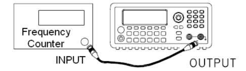
2. Set the instrument to the output described in the table below and measure the output frequency. Be sure the instrument output is enabled.
